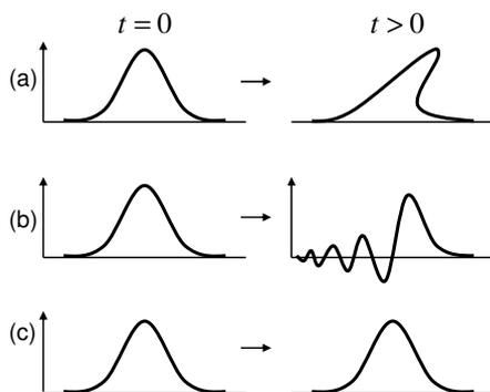
Fig. 4. Nonlinear and dispersive soliton behaviour: (a) nonlinear term only; (b) dispersion term only; (c) nonlinear and dispersion terms balanced together.
