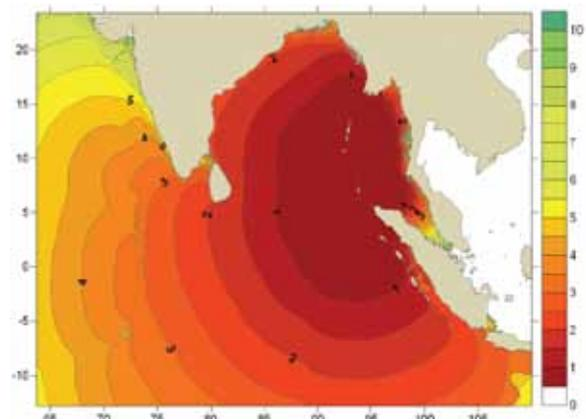
Fig. 7. Arrival time of first wave computed for the 2004 Indian Ocean Tsunami [4].
