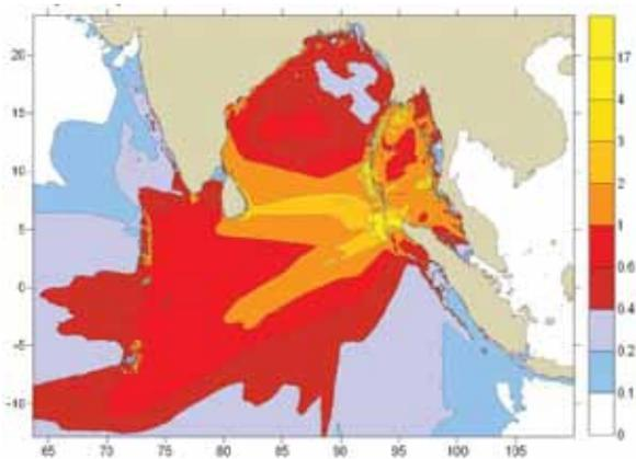
Fig. 6. Maximum wave height computed for the 2004 Indian Ocean Tsunami [4].
